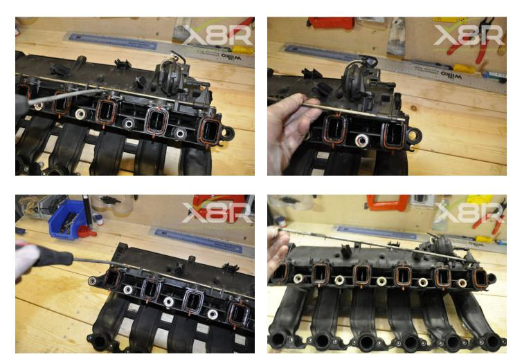
Step 10: Remove swirl flaps - Remove the swirl flaps by unscrewing the two torx bolts holding each one and lever out of position.
