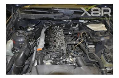
Step 8: Removing the swirl flaps - Remove the red rectangle shaped rubber seals and clean them
