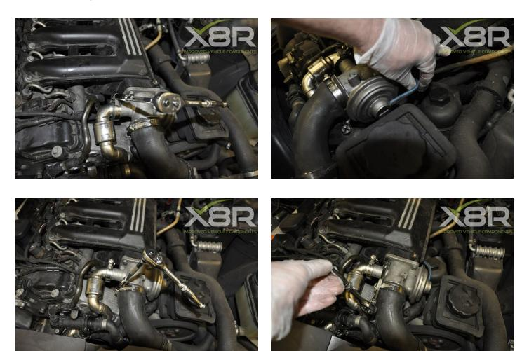
Step 6: Remove manifold - Remove the intake manifold by opening 12 bolts and 7 nuts
