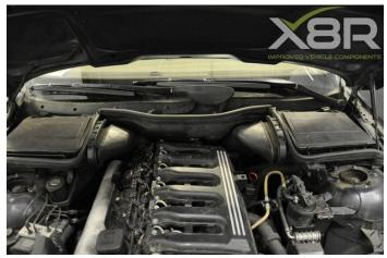
Step 3: Remove particle filters and trim - Remove the particle filter on both sides, open filter cover and remove filters.
