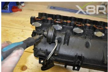
Step 9: Remove operating rod - Remove the rod by twisting it out from it's holdings. This rod does not need to be refitted as it no longer has swirl flaps to operate.
