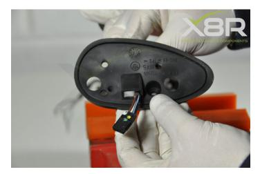
Step 5: Fit the wiring in to the new mirror base/spindle
