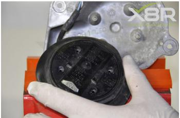
Step 4: Remove the wiring from the mirror spindle and base.
