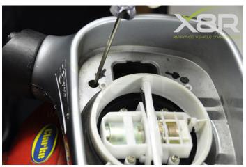
Step 8: Fit the mirror glass and base seal
