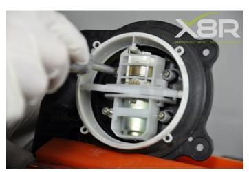
Step 7: Fit the wing mirror cover Lay the back mirror cover down, slot the spindle in the cover making sure the tabs on the cover line up.
