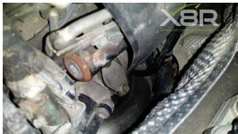
Step 6: Remove butterfly from actuator shaft in butterfly housing
