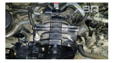
Step 7: Remove stub pipes
