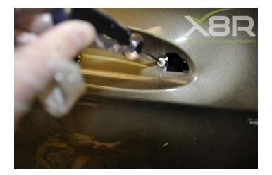
Step 4: Release actuator Remove the 3x Torx screws holding the actuator.
