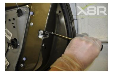
Step 5: Remove metal plate Drill out rivets and remove metal plate. 8 Rivets in total located around the edge of the metal plate.
