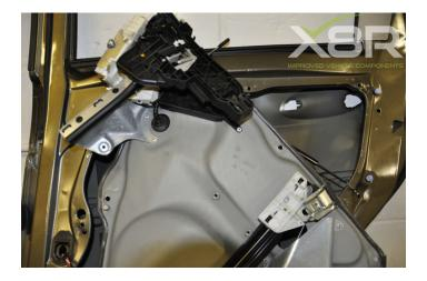
Step 6: Remove actuator Release electrical connector, linkage and trim to remove actuator from metal plate.
