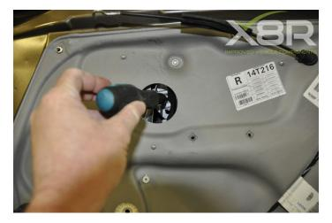
Step 3: Remove outer door handle Remove blanking plate and unscrew torx holding outer door handle.
