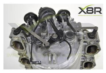
Step 1: Remove lever arms and actuator arm ball joint
