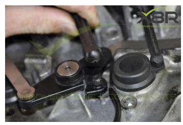
Step 2: Remove lever bolt and remove lever Using a T30 Torx screwdriver remove the bolt retaining the lever.
