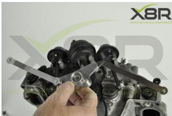
Step 3: Grease the ball joints on the new lever and arms
