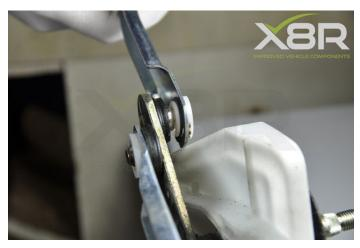
Step 8: Refit the linkage to the vehicle
